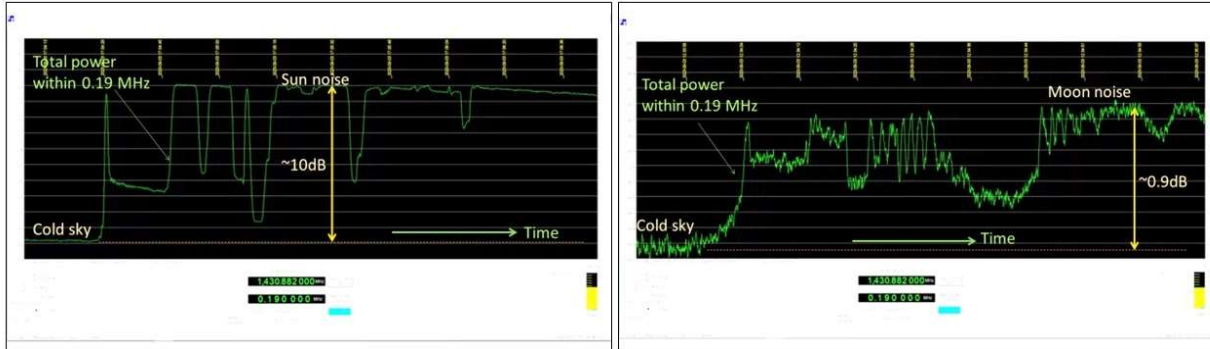
Figure 52 – Sun and Moon noise detected by my X-band system using the 3.5 m antenna. These measurements are excellent for benchmarking against other systems. These measurements show that my 3.5m dish underperforms for a dish of this size.
