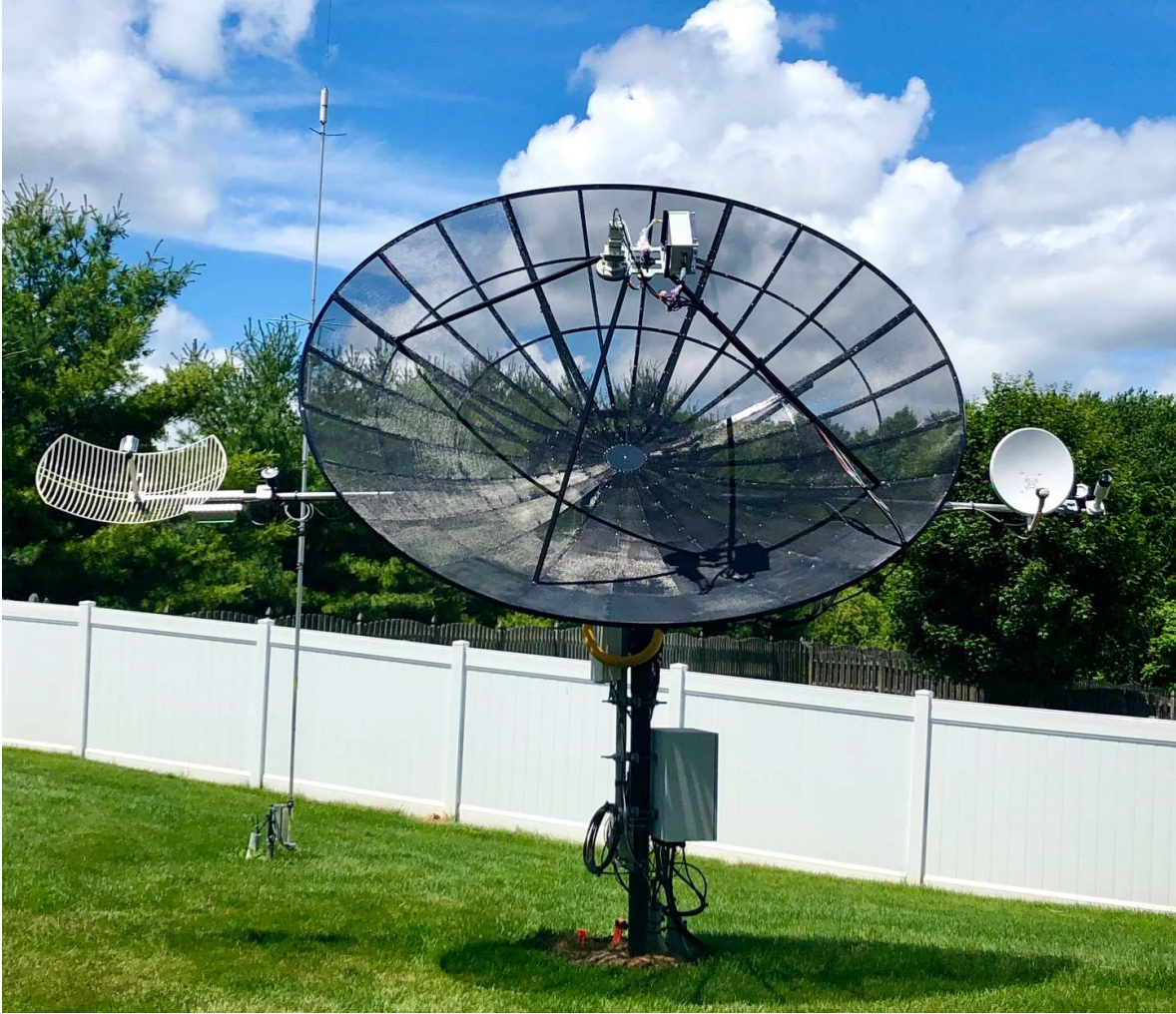
Figure 17 – 3.5m mesh dish with X-band feed and N2QG downconverter mounted on the feed-point bracket.
