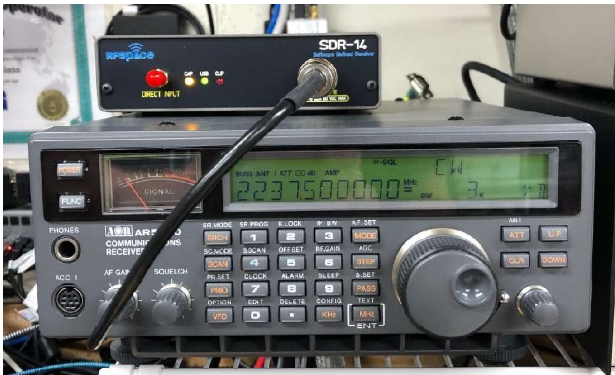
Figure 42 – My AOR AR-5000 receiver and the RFspace SDR-14 that I use for IF sampling.
