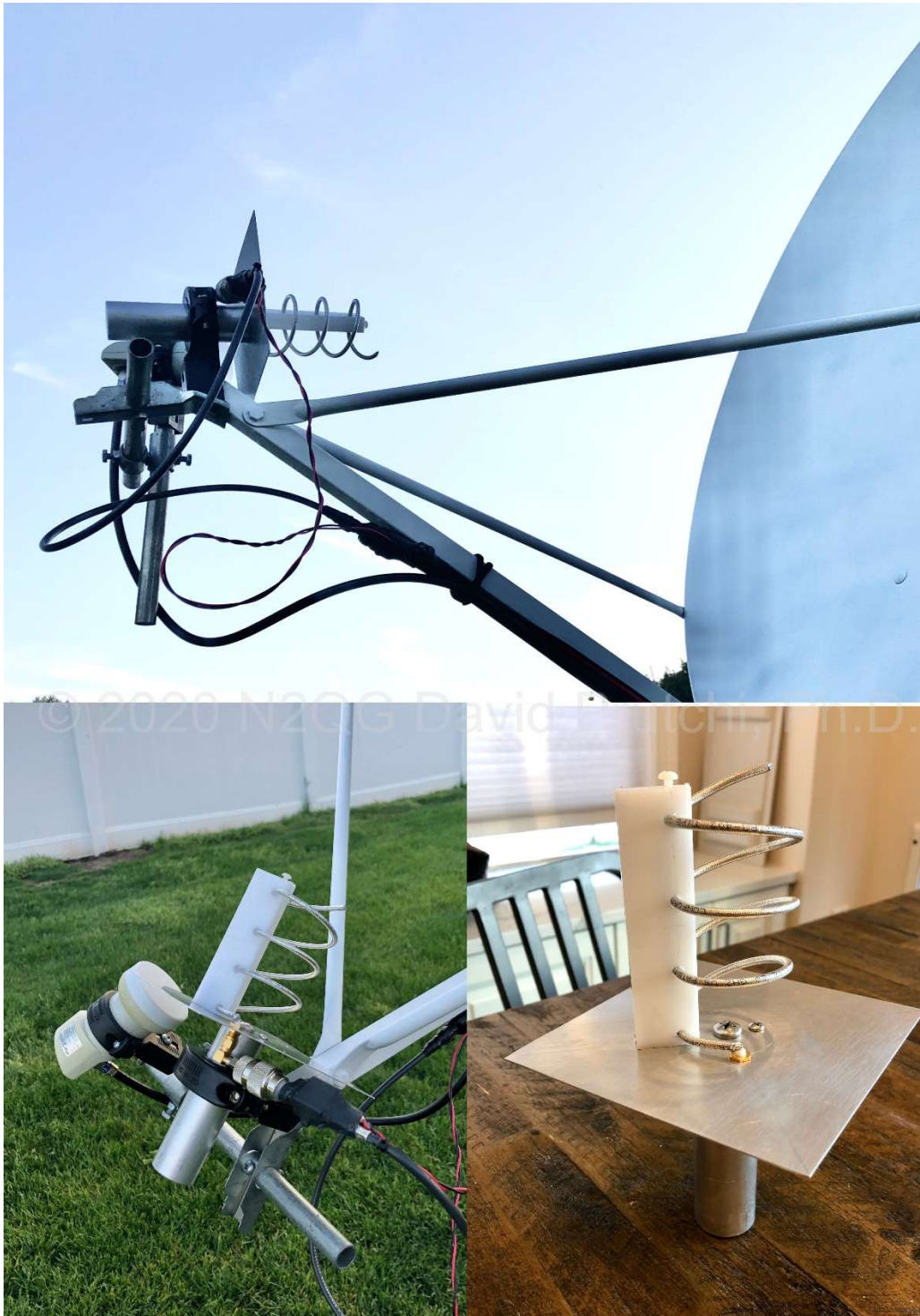
Figure 22 – My S-band feed for the 1.2m offset dish is a home-built 3.5-turn helical antenna
