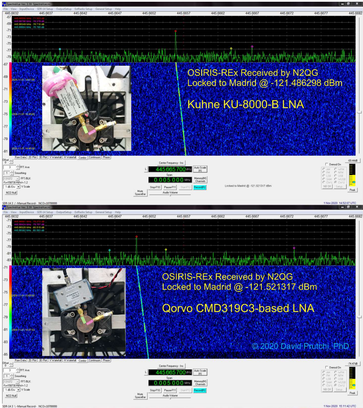
Figure 35 – Comparison of signals received from the same spacecraft using Kuhne KU-8000-B LNA versus homebrew LNA based on Qorvo CMD319C3.
