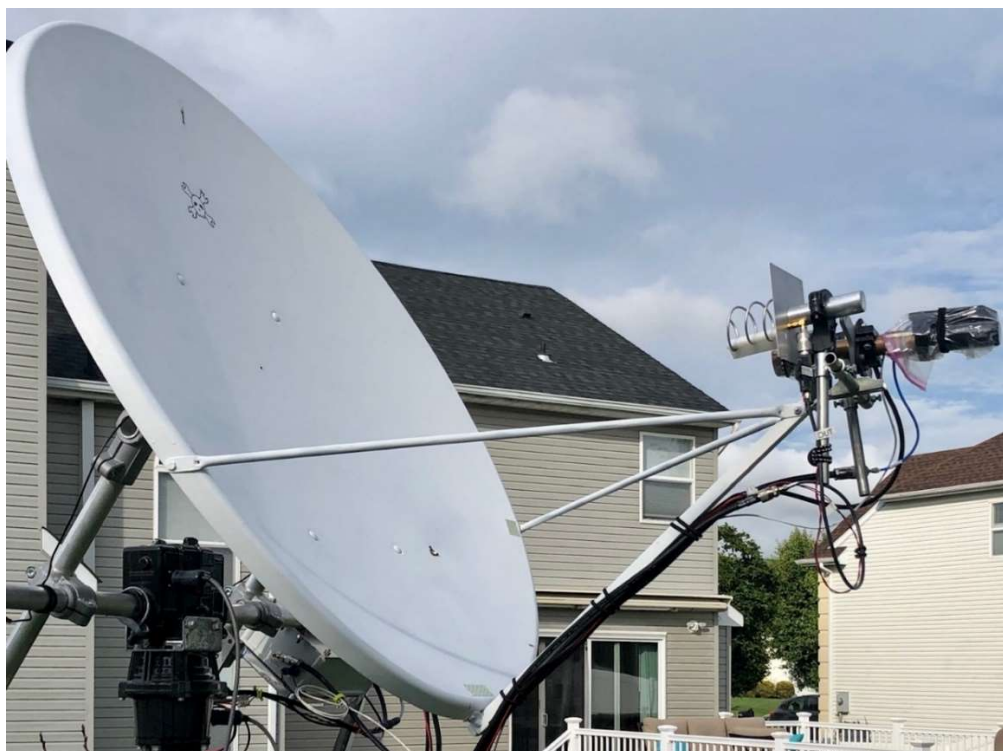
Figure 15 – Fortec Star 1.2m, f/d=0.6 offset dish shown with S-, X-, and Ku-band feeds
