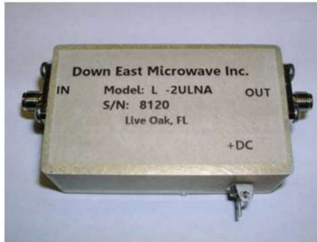
Figure 36 – Low-cost, high-performance LNA suitable for amateur DSN work.
