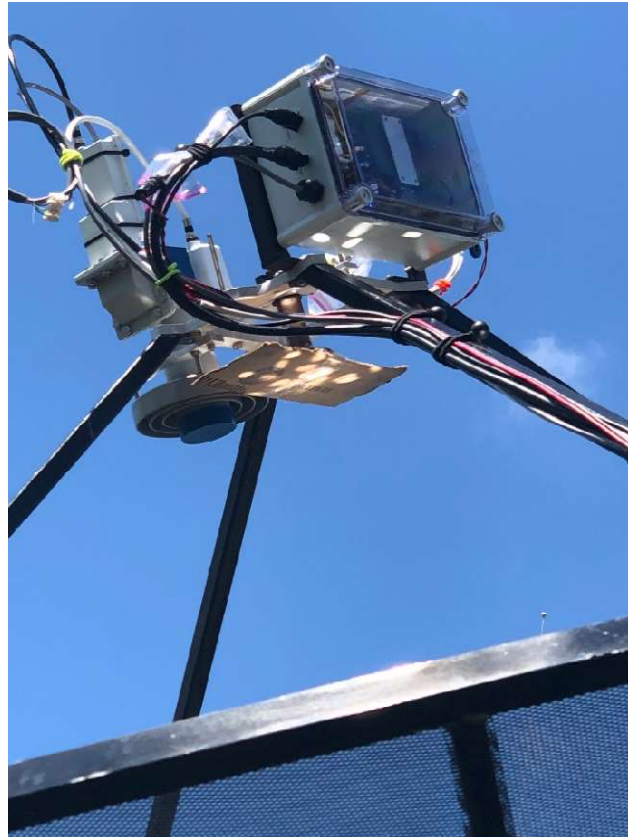
Figure 20 – Evaluating surface accuracy with small mirrors attached to the reflector shows spread at the focal point.
