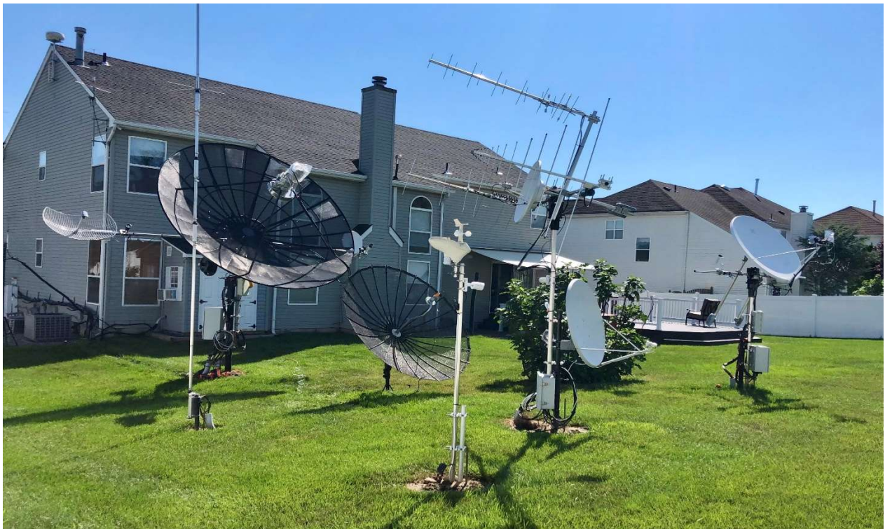
Figure 1 – Antennas at my QTH. I commonly use the 3.5m and 1.2 m dishes mounted on Az/El rotators for Amateur DSN
