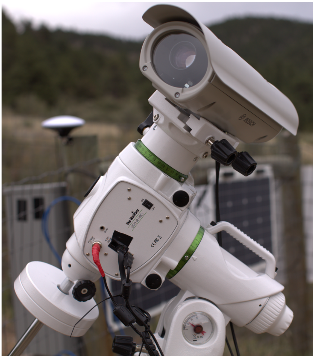
Figure 4.1: SatNOGS-Optical ground station prototype.
