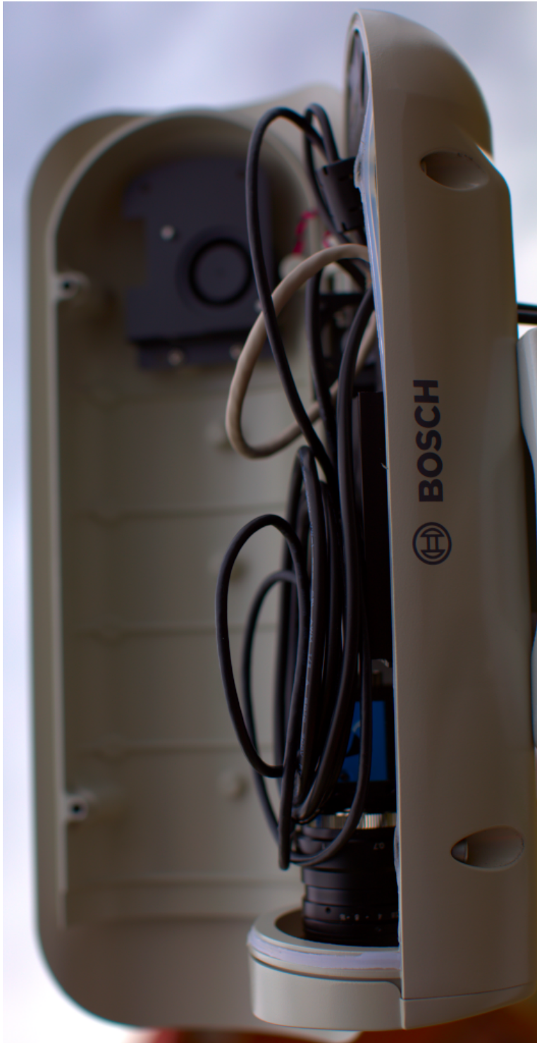
Figure 4.5: Camera enclosure, right side, opened.
